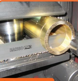
**Combo** - New tooth geometry with variable teeth 8-10° rake angle makes the 3851 toothing more robust and increases the performance.
