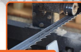
**Hook** - Traditional tooth design with 10° rake angle, used for non-ferrous metals, wood and plastics.
