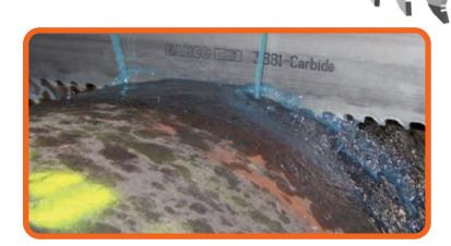
**THS** - Multi-chip tooth is designed for cutting Inconel and Waspaloy. It is wide set as standard, where pinching is a problem and produces smaller chips to reduce cutting forces and increase life. Applications in medium to large size materials with scale.
