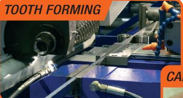
High technology milling and grinding processes are used for precision tooth forming, enabling the production of sharper and stronger teeth.
