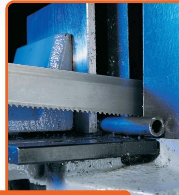
**EZ** - This patented design gives a very versatile blade, able to cut all common materials in addition to being very resistant to tooth stripping. Ideal for small workshops cutting different sizes in a wide range of materials.
