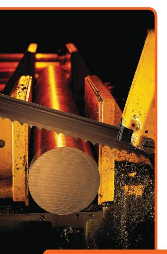
**Combo** - Traditional shape tooth with varing degree, 8° or 10° rake angle makes M42 suitable for multipurpose cutting of thin-walled tubes and profiles in most materials.
