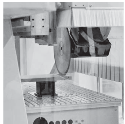
Groove cuts on CNC machining center. WOCHNER carries out inclined cuts.
