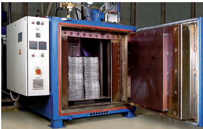
Anlassofen · Tempering furnace
