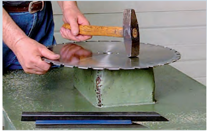
Feinrichten · High-precision straightening of the blades
