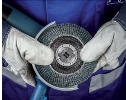
Lightly press the disc down until it audibly clicks into place.
