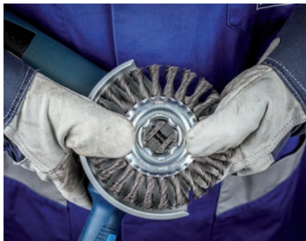
Lightly press the brush down until it audibly clicks into place.
