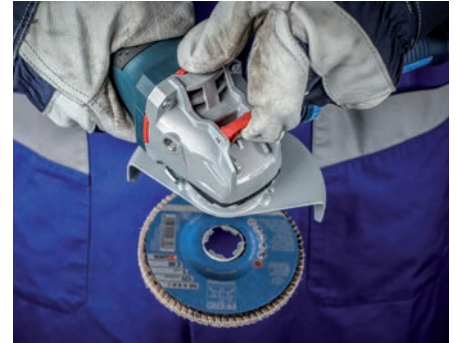
Release the disc by using the lever.
